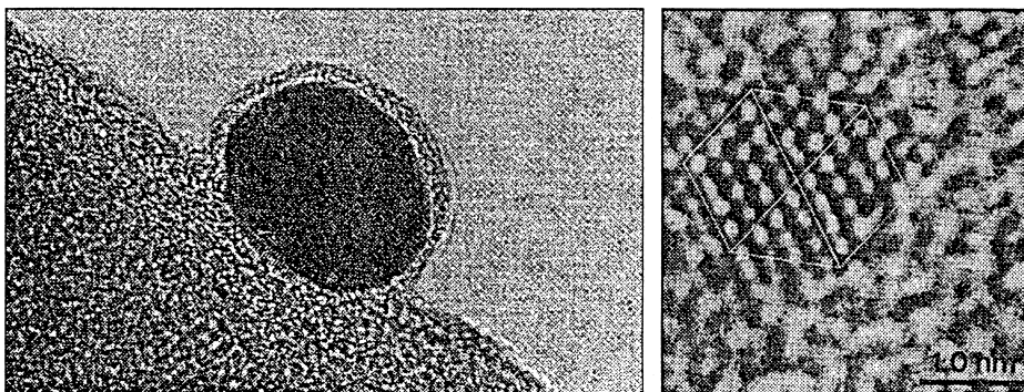
Fig. 6. Left, HR-TEM image of a 132 \times 105 \text{ \AA} gold colloid surrounded by two layers of \text{P}(m\text{-C}_6\text{H}_4\text{SO}_3\text{Na})_3 stabilizing ligands. Right, HR-TEM image of a \text{Pt}_{309} cluster molecule in the (110) direction showing nine rows of the fcc structure, corresponding to a four-shell cluster. Both images are from Ref. [109].
